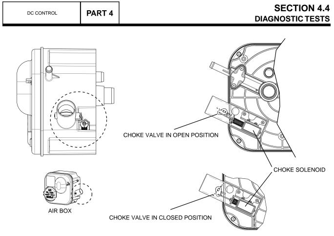
Figure 26. 8kW Choke Solenoid
